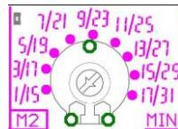
The “MIN” trimmer is used to adjust the minimum motor current for protection against the risk of dry run, for added protection or when minimum level floats or probes are not required.
